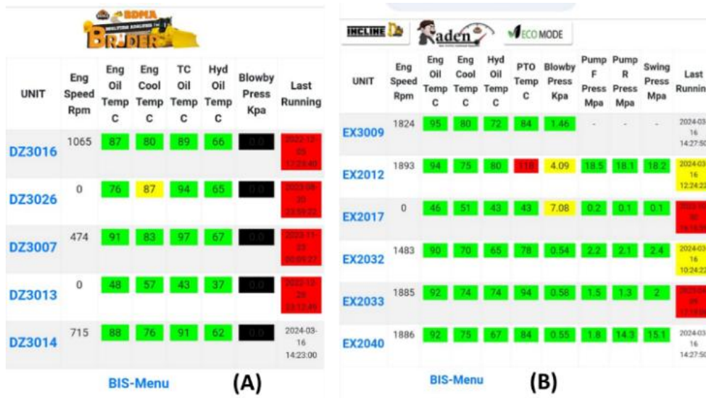
Figure 6. Mobile view of real-time temperature monitoring dashboard for units: D375A (A), PC1250-8 and PC2000-8 (B)
