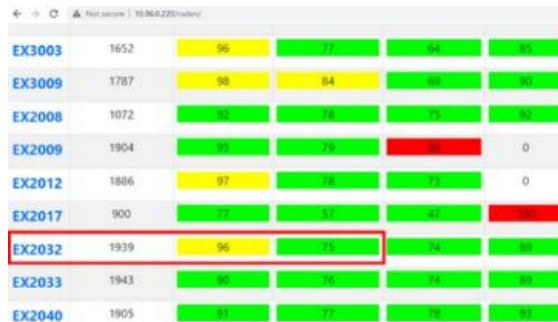
Figure 9. Dashboard showing EX2032 (PC1250-8) to have engine oil and coolant temperature different more than 20°C
